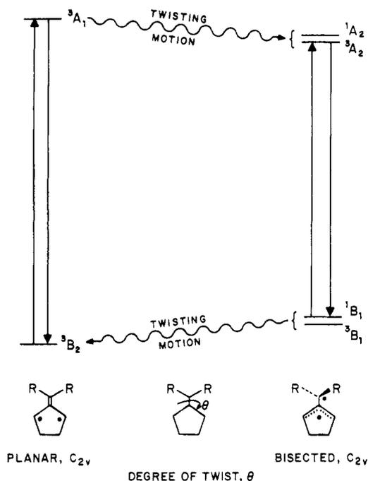
**Figure 4.** Schematic diagram of the interconversion of trimethylmethane species. Planar and bisected geometries are shown as specific possibilities.
