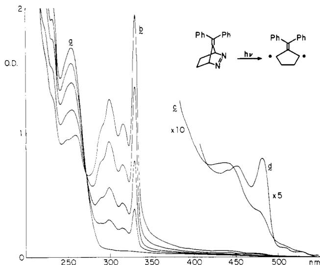
**Figure 1.** UV/vis spectra recorded during stepwise photolysis of **2a** at 79 K (a) before photolysis (Initial concentration in MCH at 300 K:  $1.1 \times 10^{-3}$  M). (b) same after a total of 290 s exposure ( $\lambda$  254 nm) (Intermediate spectra shown). (c) same after 560 s exposure (expanded 10 $\times$ ). (d) spectrum (expanded 5 $\times$ ) after 86 min photolysis of a  $1.1 \times 10^{-2}$  M solution of **2a** in EPA.
