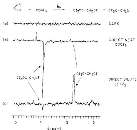
Figure 1. The  $^1H$ -NMR spectra (80 MHz) of diazirine in (b) neat chloroform-d and (c) in  $C_6F_{14}$  containing saturated  $CDCl_3$  upon direct photolysis ( $>300$  nm). A spectrum of the same region after irradiation is shown in (a).
