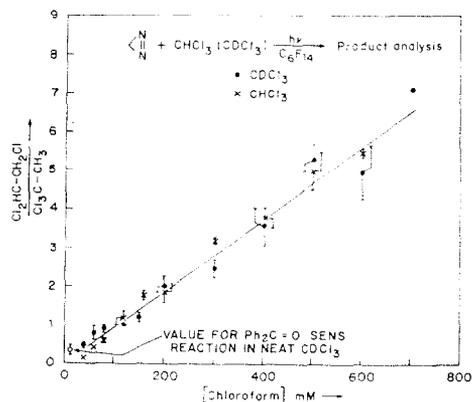
Figure 2. The ratio of the  $Cl_2HC-CH_2Cl$  yield to the  $Cl_3C-CH_3$  yield from the photolysis of diazirine with various concentrations of chloroform (x) or chloroform-d (●) in  $C_6F_{14}$  solution at  $0^\circ C$ . (○) represents benzophenone triplet decomposition of diazomethane in neat  $CDCl_3$  at  $0^\circ C$ .
