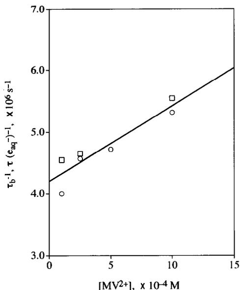
Fig. 5. Dependence of  $[MV^{2+}]$  on the decay rate constant of  $e_{aq}^-$ ,  $\tau(e_{aq}^-)^{-1}$  (□), and growth rate constant of  $MV^{+\cdot}$ ,  $\tau^{-1}$  (○).
