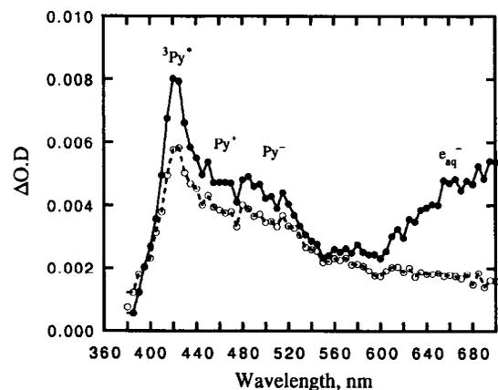
Fig. 1. Transient absorption spectra obtained for Py-PPC ( $n=9$ ) in a DPPC vesicle solution in the absence of methylviologen at two times after laser excitation. Py-PPC:DPPC = 1:29. ( $\bullet$ , —) 0.82  $\mu\text{s}$ ; ( $\circ$ , ---) 8.1  $\mu\text{s}$ .
