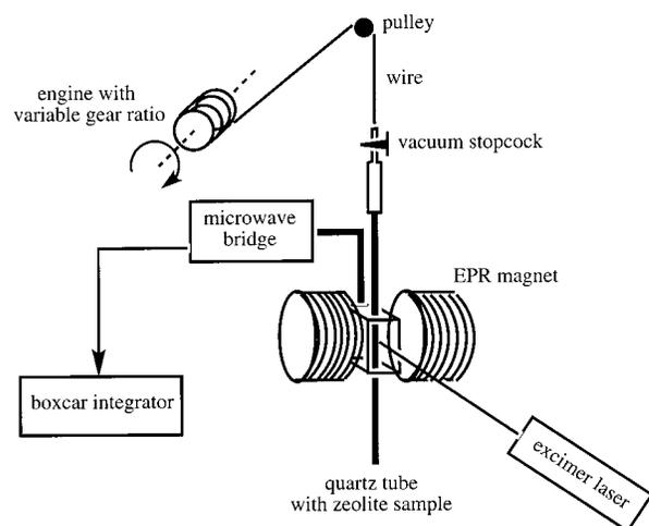
**Figure 1.** Schematic representation of the instrumentation used to measure electron spin polarization in powder samples by TR-EPR.
