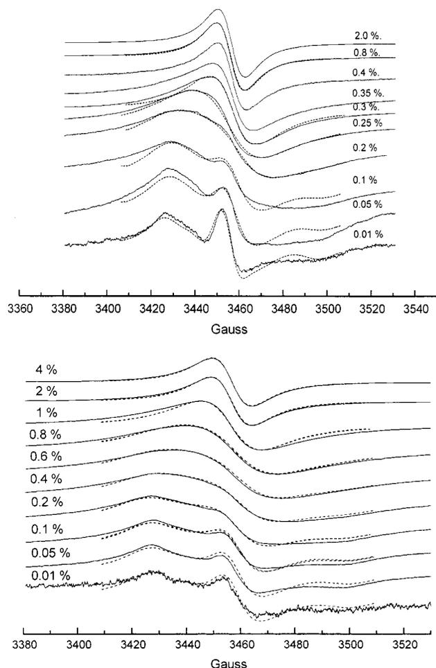
**Figure 1.** (a) EPR spectra of **1** on silicalite at various loadings, indicated at the right of the spectra. The solid lines are experimental results and the dashed lines are from computational simulations. (b) EPR spectra of **1** on LZ-105 at various loadings, indicated at the left of the spectra. The solid lines are experimental results and the dashed lines are from computational simulations.
