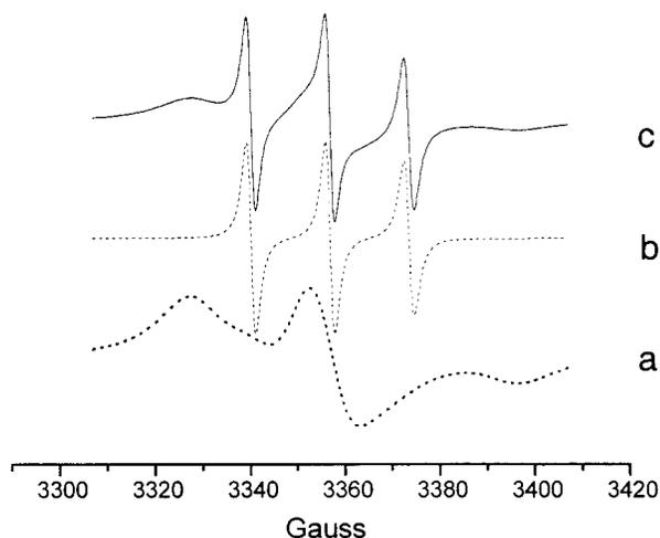
**Figure 5.** Addition of EPR spectra at slow motion and fast motion to reproduce an experimental spectrum. (a) spectrum computed for slow motion, (b) spectrum computed for fast motion. (c) result from addition of (a) and (b), to produce a good fit to the experimental spectrum.
