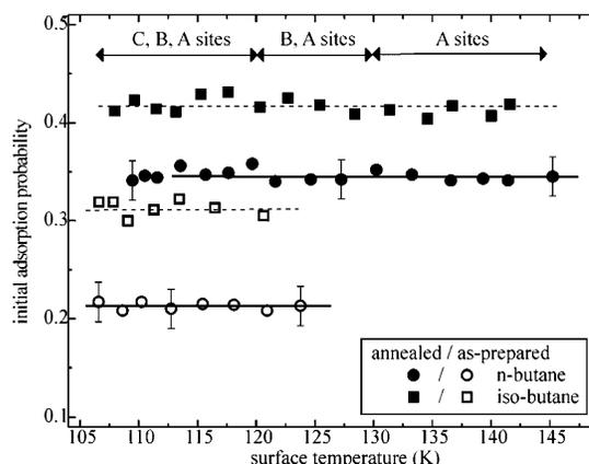
**Figure 5.** Temperature dependence of the initial adsorption probability of *n*-/isobutane adsorbed on the CNTs (annealed/as-prepared). ( $E_i = 0.74$  eV for *n*-butane, and  $E_i = 0.31$  eV for isobutane.) The arrows indicate the temperature range where the different adsorption sites on the CNTs are kinetically favored.
