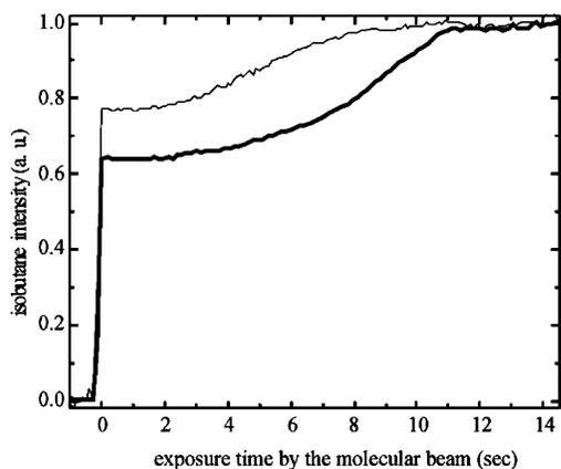
**Figure 3.** Example of adsorption transients, that is, the isobutane pressure in the scattering chamber of the beam system versus exposure time by a 3% isobutane beam (balance He) is shown. The thick solid line is for o-CNTs ( $E_i = 0.74$  eV); the thin solid line is for c-CNTs ( $E_i = 0.85$  eV). The transients normalized as  $1 - \text{adsorption probability}$  versus exposure time are shown ( $T_{\text{ads}} = 112$  K).
