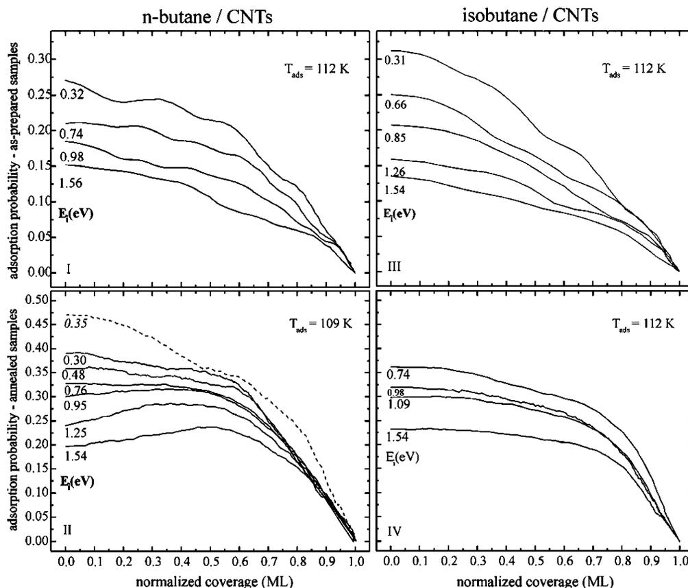
**Figure 6.** Coverage dependence of the adsorption probability parametric in impact energy,  $E_i$ , and at an adsorption temperature just above the condensation temperature of the alkanes, as indicated. Left column: *n*-butane. Right column: isobutane data. Top row: as-prepared CNTs. Bottom row: annealed CNTs. (The dashed line in panel II is for *n*-pentane adsorption at  $T_{\text{ads}} = 135$  K.)
