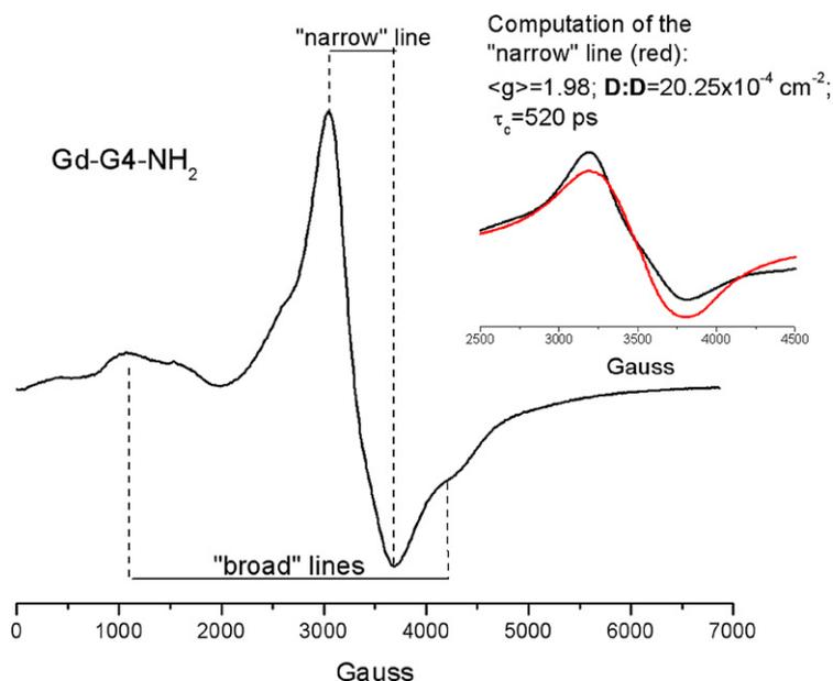
**Fig. 1.** EPR spectrum of Gd-G4-NH<sub>2</sub> dendrimer in solution recorded in the 0–7000 G range at 298 K. The two spectral components are indicated in the spectrum as “broad” and “narrow” lines. In the insert the computation of the “narrow” line is shown.
