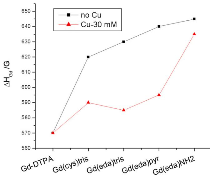
**Fig. 2.** Variation of the line width of the EPR spectrum of the Gd-G4-dendrimers in the absence and in the presence of  $\text{Cu}^{2+}$  (30 mM).
