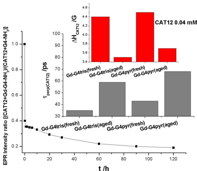
**Fig. 4.** Variation over time after sample preparation of the relative intensity of the EPR signal of CAT12 in solution (0.04 mM) in the presence of Gd-G4-NH<sub>2</sub>. The insert in the figure compares the  $\tau_{\text{perp}}(\text{CAT12})$  and  $\Delta H_{\text{CAT12}}$  parameters for the freshly prepared and the aged (1 day) samples containing CAT12 and Gd-G4-tris or Gd-G4-pyr.
