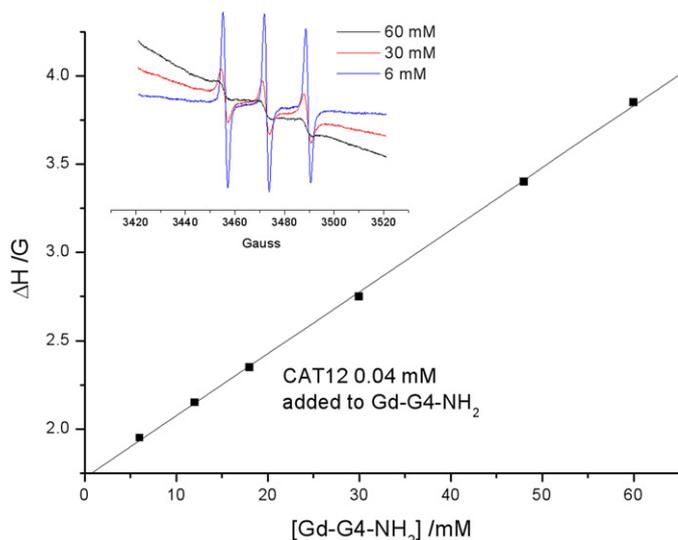
**Fig. 3.** Variation of the line width of the EPR spectrum of CAT12 (0.04 mM, at 273 K) as a function of the concentration of Gd-G4-NH<sub>2</sub>. The insert in the figure shows some representative spectra of this system at [Gd-G4-NH<sub>2</sub>] = 6, 30, and 60 mM.
