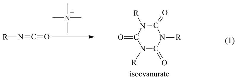
Formation of isocyanurate in the case of common diisocyanates TDI and IPDI was demonstrated by IR, with characteristic peaks at 1695–1715 cm<sup>-1</sup> [29]. Polyol with dispersed organoclay and diisocyanates transforms into a solid or a very viscous
