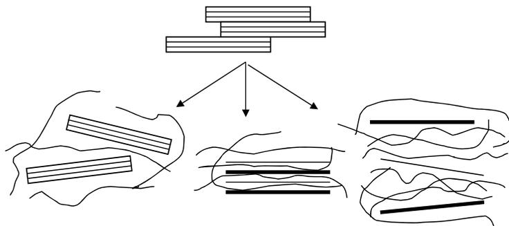
**Figure 1.** A common pictorial presentation of three types of polymer composites with clay (top). Bottom left, conventional composite; bottom center, intercalated nanocomposite; bottom right, exfoliated nanocomposite. After Refs [3, 8, 9].
