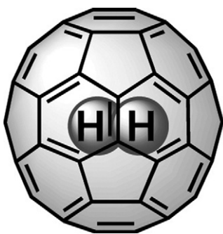
Fig. 1. Structure of the \text{H}_2@C_{60} supramolecular complex.
