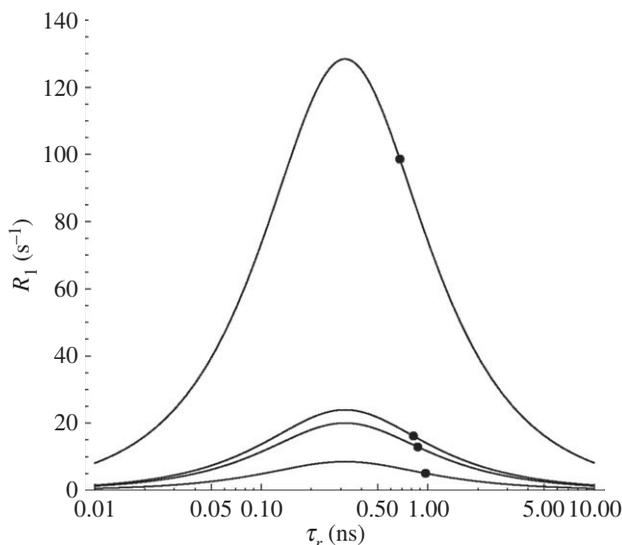
**Figure 7.** Plots of equation (2.3) as a function of  $\tau_c$ . Each curve (highest to lowest) corresponds to the value of  $r_{S1}$  calculated for molecules **1–4**. Other parameters:  $S = 1/2$ ;  $g_e = 2.0067$ ;  $\omega_I = 500$  MHz. All curves go through a maximum for  $\tau_c = 0.318$  ns. Dots correspond to the calculated correlation times with stick boundary conditions (table 1).
