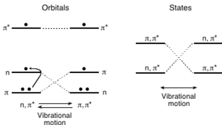
**Figure 5.4** *Orbital and state descriptions of  $n,\pi^* \leftarrow \pi,\pi^*$  state switching as a result of vibrational motion.*
