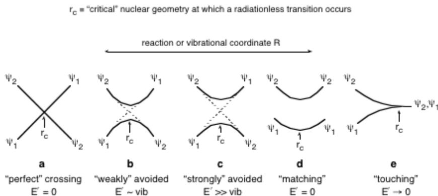
**Figure 5.2** *The archetype adiabatic surface topologies for a two surface system: (a) “perfect” crossing for which  $\Psi_1 \rightarrow \Psi_2$  transitions are strictly forbidden; (b) and (c) “weakly” and “strongly” avoided crossings for which  $\Psi_1 \rightarrow \Psi_2$  transitions are possible near  $r_c$  (see text); (d) “matching” for which  $\Psi_1 \rightarrow \Psi_2$  transitions are very improbable (see text).*
