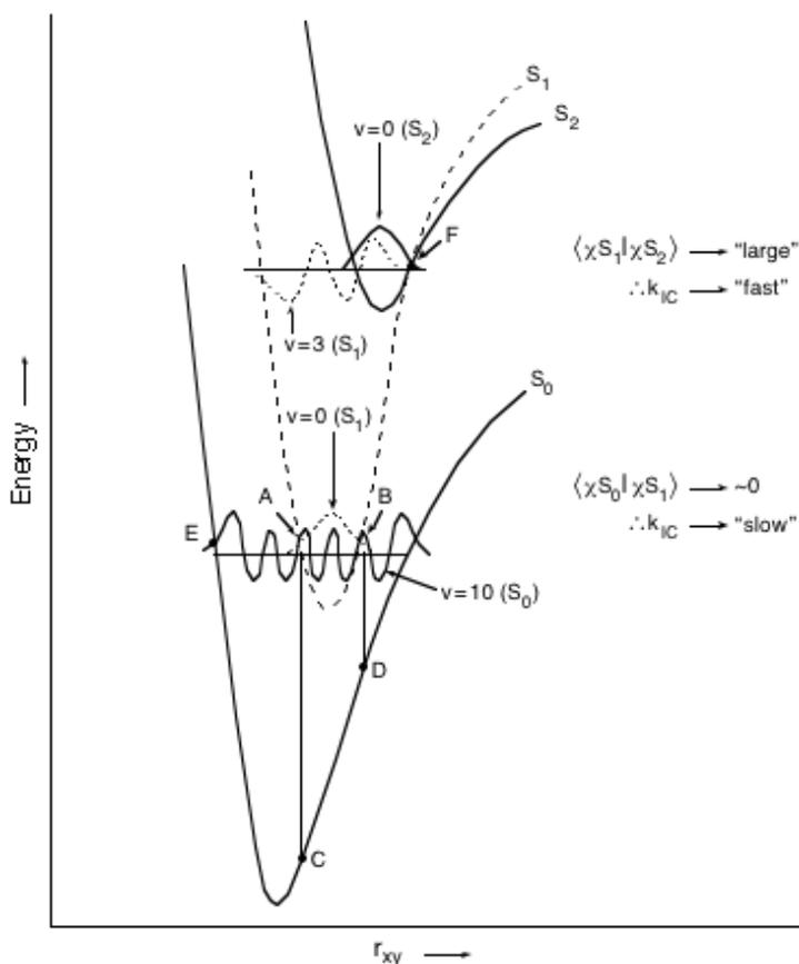
**Figure 5.13** Representation of internal conversion between  $S_2$  and  $S_1$  and between  $S_1$  and  $S_0$ .
