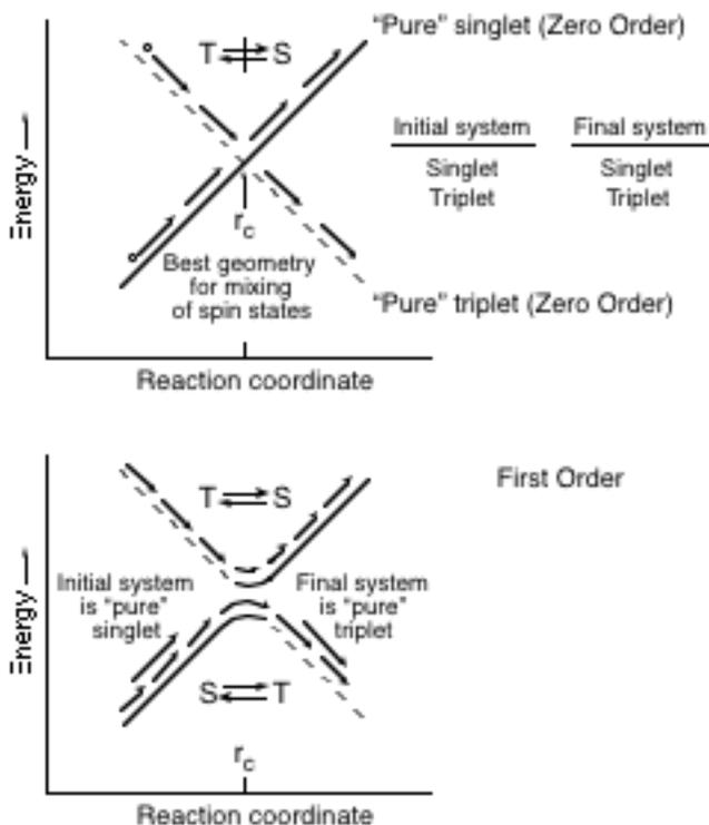
**Figure 5.7** Intersystem crossing is strictly forbidden in the Zero Order approximation (top figure) but becomes partially allowed when a spin mixing mechanism is available (lower figure).
