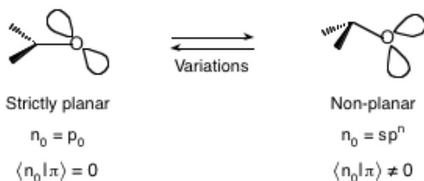
**Figure 5.5** Schematic of the "mixing" of  $s$  character into a  $p$ -orbital as the result of nonplanar vibrations.
