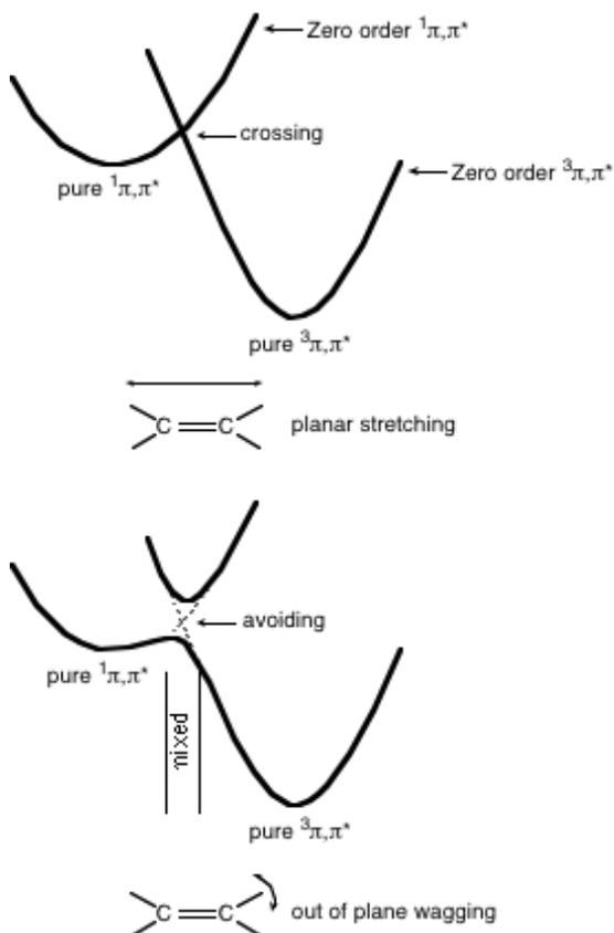
**Figure 5.11** *Vibronic interactions. Top: planar vibrations do not mix states, so that a Zero Order crossing persists in First Order. Bottom: out-of-plane vibrations cause an avoiding.*
