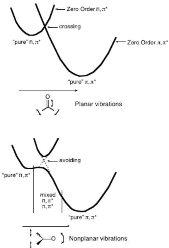
**Figure 5.6** The effect of planar (top) and nonplanar (bottom) vibrations on a Zero Order crossing of  $n, \pi^*$  and  $\pi, \pi^*$  surfaces.
