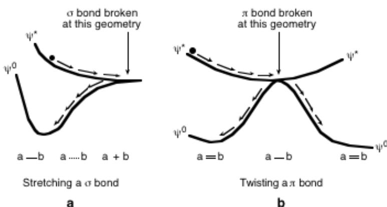
**Figure 5.12** Schematic representation of (a) the stretching of a  $\sigma$  bond and (b) the bending of a  $\pi$  bond.
