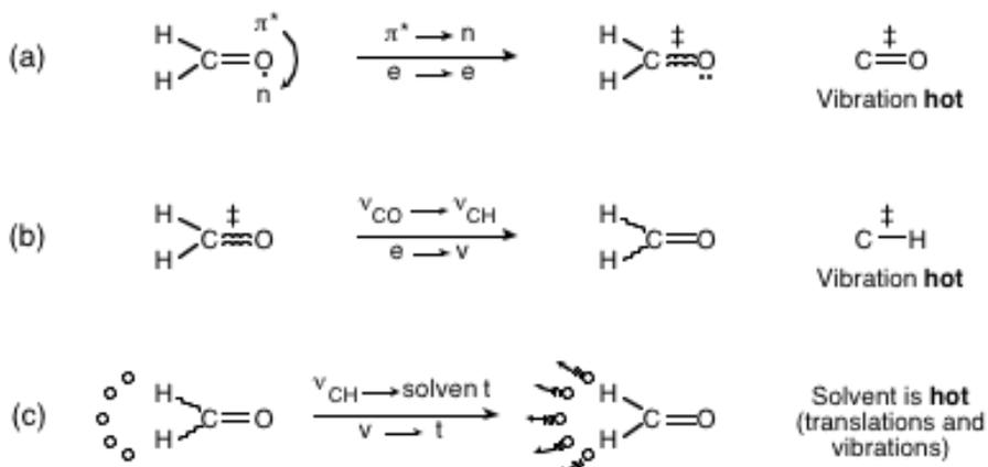
**Figure 5.14** Schematic description of energy dissipation for formaldehyde. (a) the conversion of electronic excitation into vibration for formaldehyde, initially localized as excitation (wiggly lines) between the C and O atoms, followed by (b) vibrational energy transfer to the CH bonds, and (c) transfer to translational motion of the solvent.
