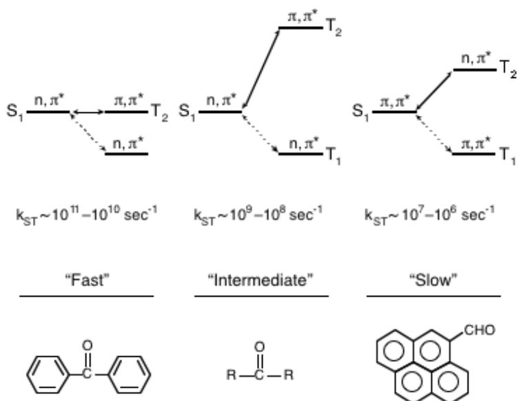
**Figure 5.10** Examples of different rates of intersystem crossing for  $S_1(n,\pi^*) \rightarrow T(\pi,\pi^*)$ ,  $S_1(n,\pi^*) \rightarrow T(n,\pi^*)$  and  $S_1(\pi,\pi^*) \rightarrow T(\pi,\pi^*)$ , of carbonyl compounds.
