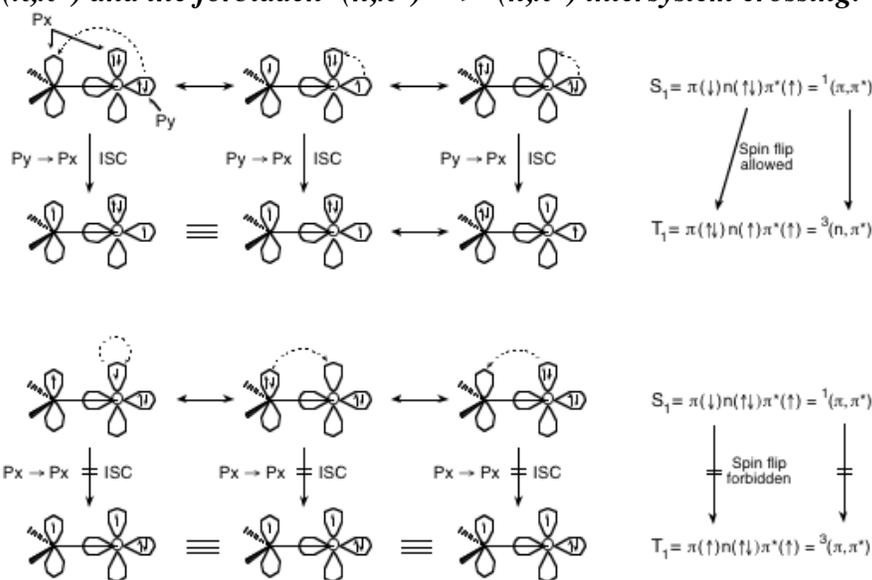
**Figure 5.9** Qualitative orbital description of the allowed  ${}^1(\pi, \pi^*) \rightarrow {}^3(n, \pi^*)$  and the forbidden  ${}^1(\pi, \pi^*) \rightarrow {}^3(\pi, \pi^*)$  intersystem crossings.
