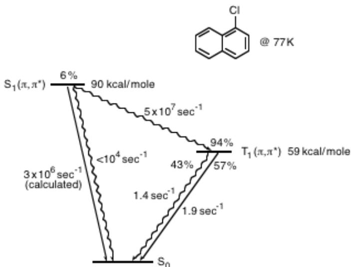
**Figure 5.15** Energy diagram for 1-chloronaphthalene at 77 K, at 25° C,  $k_1 \sim 10^4 \text{ sec}^{-1}$ .
