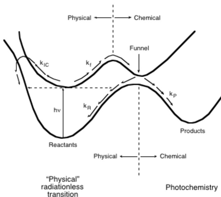
**Figure 5.17** Schematic surface description of a possible relationship between "photophysical" and photochemical radiationless processes.
