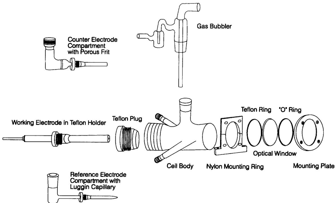
Fig. 1. The spectroelectrochemical cell and the working electrode.
