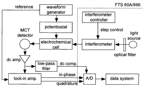
Fig. 11. Experimental setup for potential-modulated FT-IR spectroscopy
