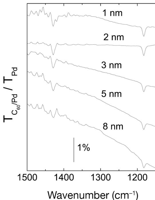
Fig. 5. Infrared absorption spectra of 30-nm-thick  $C_{60}$  as a function of the thickness of Pd on hydrogen-terminated Si(111).
