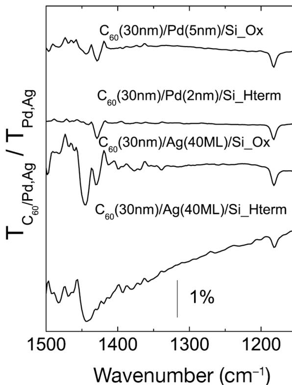
Fig. 8. The absorption spectra of 30-nm-thick  $C_{60}$  on 40 monolayer Ag deposited on surface-oxidized Si(100) and hydrogen-terminated Si(111), as compared with those of 30-nm  $C_{60}$  on the same substrates.
