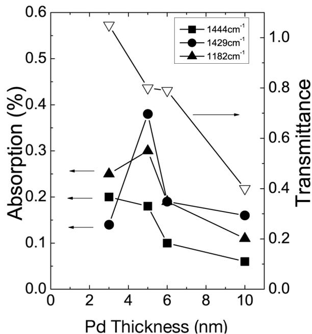
Fig. 2. Intensity changes of the  $A_g(2)$ ,  $T_{lu}(4)$ , and  $T_{lu}(3)$  modes with increasing Pd thickness (from Fig. 1). The arrow-headed lines are a visual guide only. The infrared transmittance before  $C_{60}$  deposition also changes with Pd thickness.
