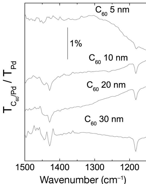
Fig. 3. The absorption spectra of  $C_{60}$  on 5-nm-thick Pd deposited as a function of  $C_{60}$  thickness deposited on surface-oxidized Si(100).
