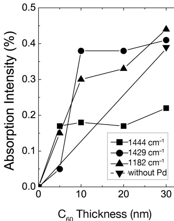
Fig. 4. Absorption intensities of the  $A_g$  (2),  $T_{1u}$  (4), and  $T_{1u}$  (3) modes versus  $C_{60}$  thickness on oxidized Si (100) (from Fig. 3). The intensity change of the  $T_{1u}$  (3) mode without Pd is also shown.
