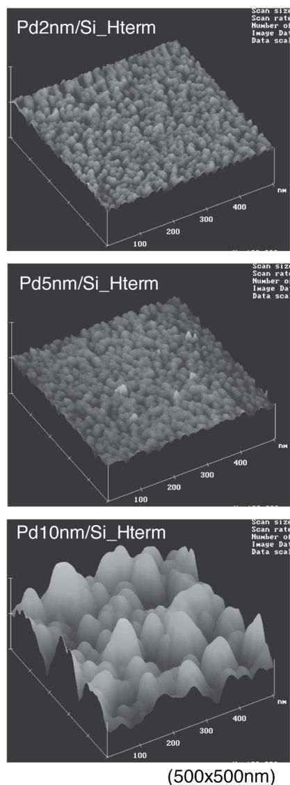
Fig. 7. AFM images of 2-, 5-, and 10-nm Pd films deposited on hydrogen-terminated Si(111)
