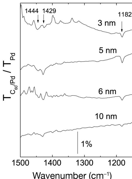
Fig. 1. Infrared absorption spectra of 10-nm-thick  $C_{60}$  as a function of the thickness of Pd deposited on surface-oxidized Si(100). The spectra are shifted vertically to avoid overlapping.
