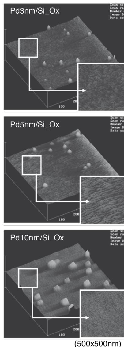
Fig. 6. AFM images of 3-, 5-, and 10-nm Pd films deposited on surface-oxidized Si(100)
