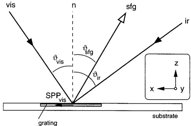
Fig. 2. Configurations for SFG with a SPP at the visible input wavelength. Left, configuration of input beams used with the prism; the SPP travels to the right, counterdirectional to the IR input beam. Right, configuration used with the grating; the SPP at the visible input wavelength is codirectional with the IR input beam.
