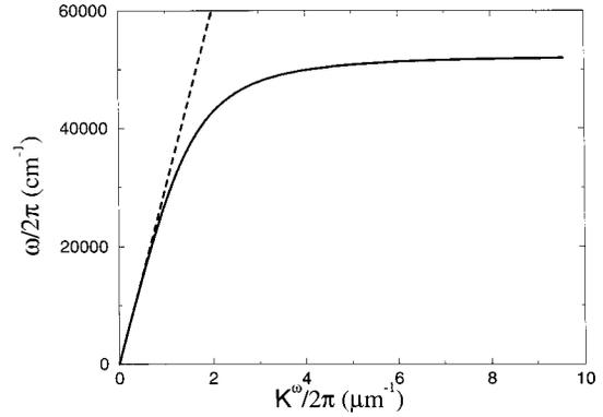
Fig. 1. Dispersion relation of a SPP propagating along the interface between vacuum and a metal (solid curve). The dashed line shows the dispersion relation of free-space electromagnetic radiation.
