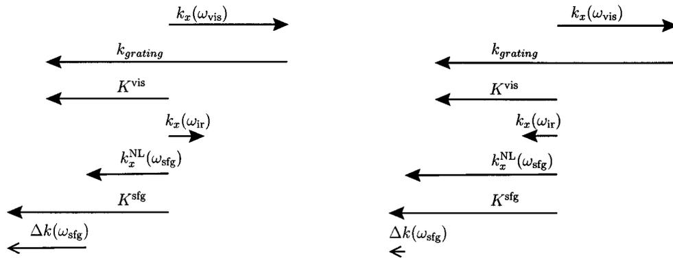
Fig. 5. Wave-vector components parallel to the interface for the grating coupler for (right) counterpropagating and (left) copropagating configurations of the input beams. The bottom arrows indicate the wave-vector mismatch for the respective cases.
