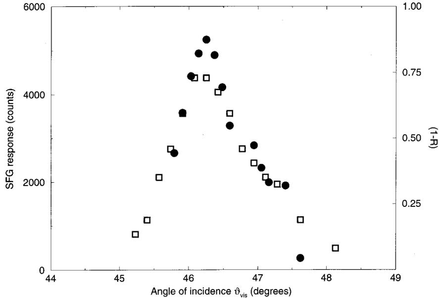
Fig. 3. Experimental results for the sum-frequency yield obtained with the prism coupler (filled symbols, scale at left). The open symbols show the fraction of the visible input power that is coupled into a polariton (scale at right).
