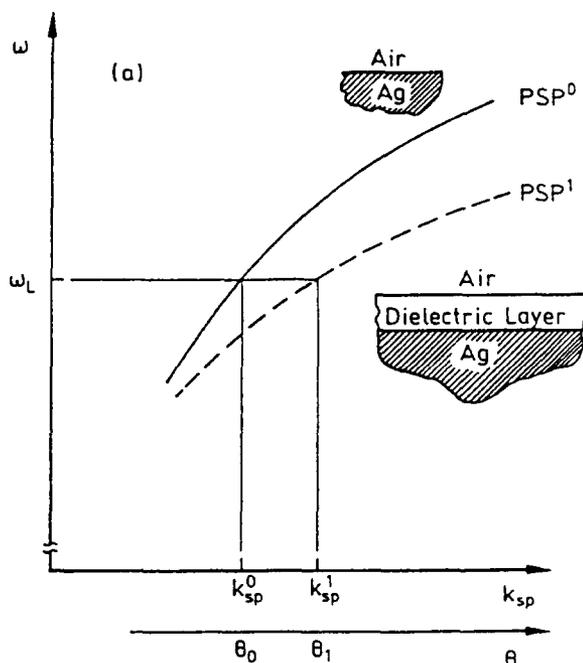
Fig. 2. Dispersion relation,  $\omega$  versus  $k_{sp}$ , of PSPs at an Ag/air-(PSP<sup>0</sup>, solid line) and at an Ag/dielectric layer/air-interface (PSP<sup>1</sup>, broken line). Laser light of an energy  $\hbar\omega_L$  couples at an angle  $\theta_0$  and  $\theta_1$ , respectively, given by the energy and momentum matching condition (horizontal line at  $\omega_L$ ).
