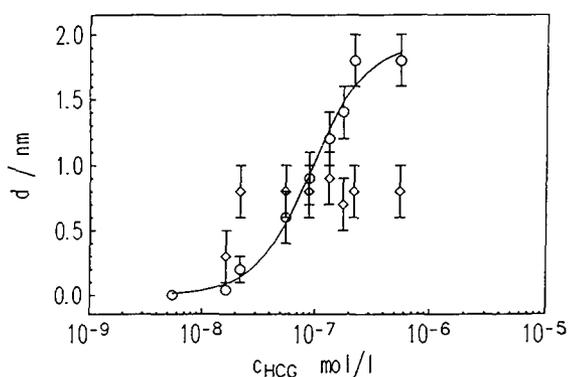
Fig. 9. Adsorption isotherm for HCG ( $\circ$ ) and subsequent adsorption of the monoclonal antibody ( $\diamond$ ) for multilayers formed with  $x_B = 0.1$ .
