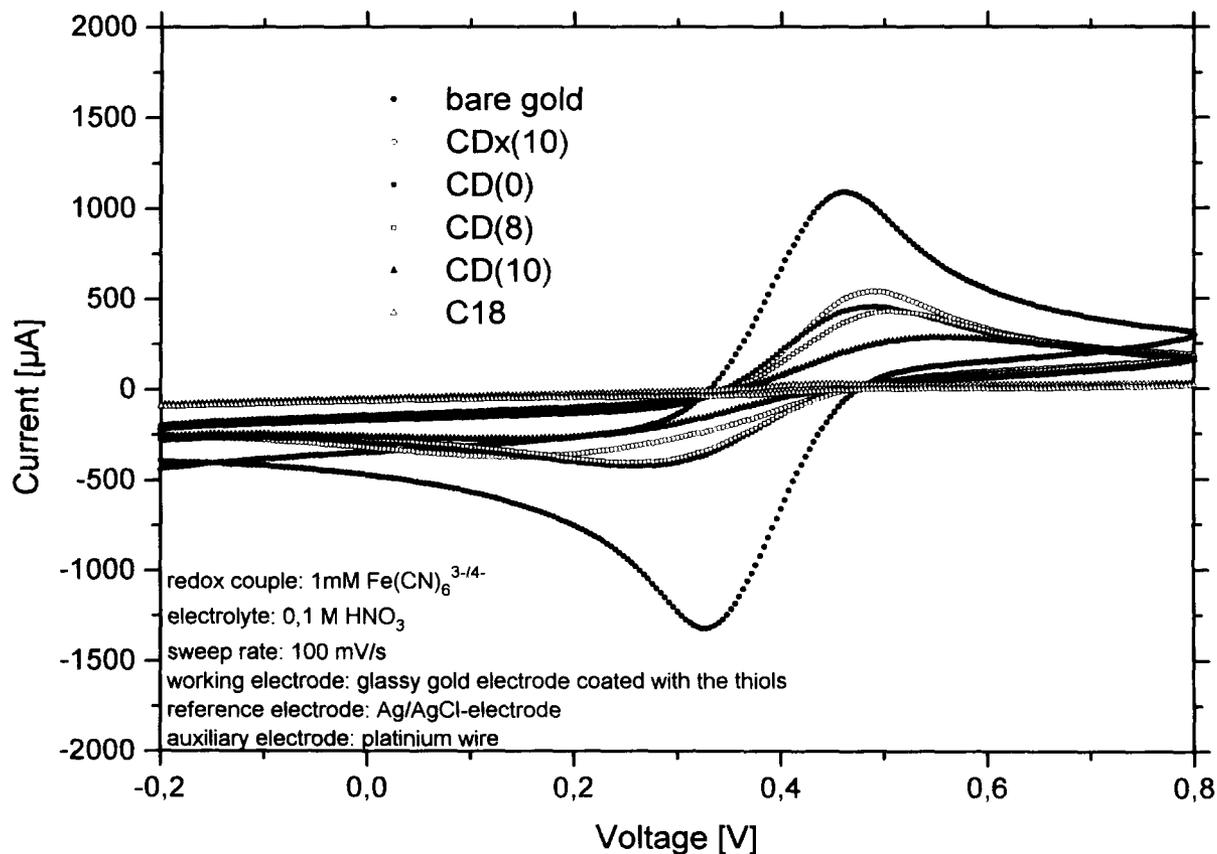
Fig. 12. Cyclic voltammograms for the pure gold surface and all four cyclodextrin derivatives. The experimental details are shown in the inset of the figure.
