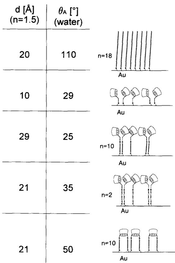
Fig. 11. Monolayer thicknesses, advancing contact angle and formation of octadecylmercaptan, CD(0), CD(8), CD(10) and CD<sub>x</sub>(10). The monolayer thicknesses and hydrophobicity indicate an elongated alkylchain with tilted cyclodextrins. The cyclodextrins with one thiol group are closely packed, whereas the multichain compound is less densely packed.
