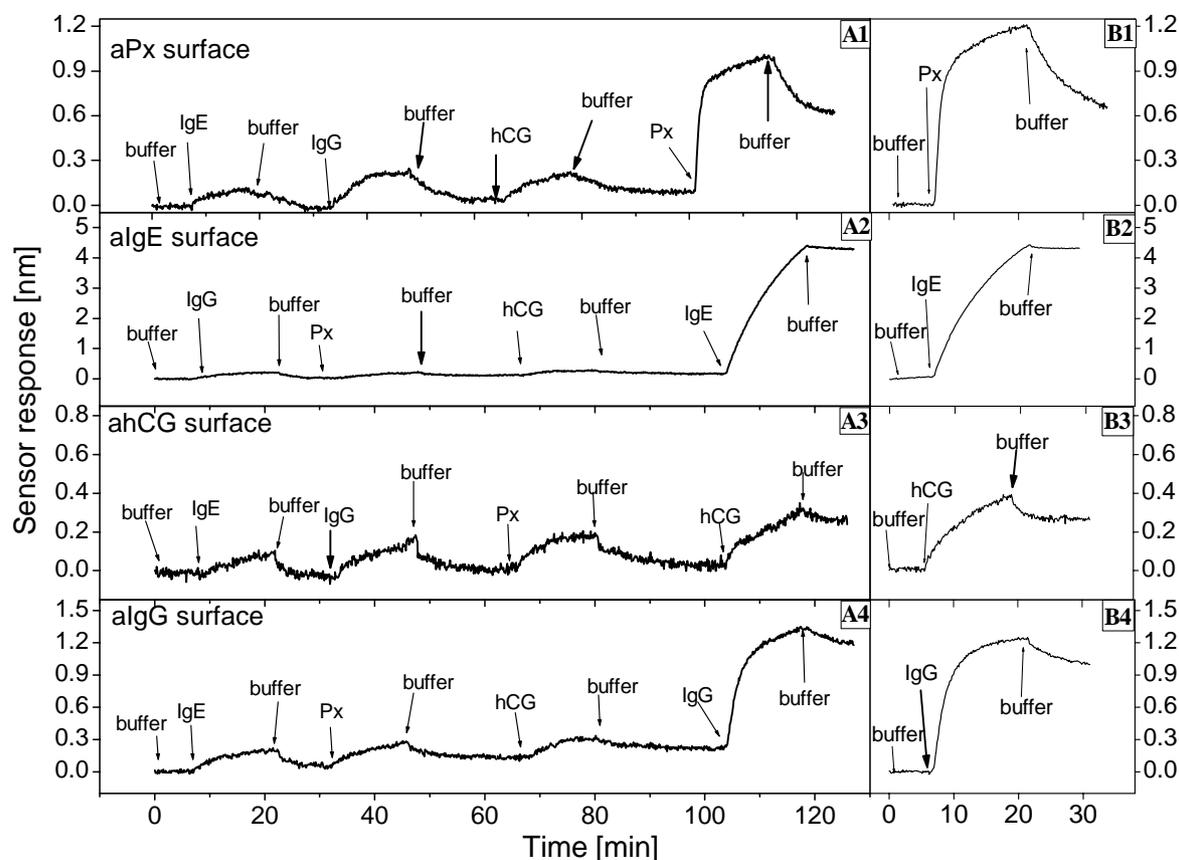
Fig. 13. Sensor response to a target analyte injected after a sequence of non-target analytes (A1–A4) and directly (channels B1–B4), concentrations of Px, IgE, hCG, and IgG are 5, 2, 2, and 5  $\mu\text{g/ml}$ , respectively.
