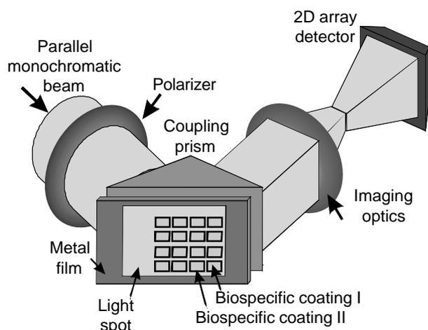
Fig. 2. SPR imaging sensor.
