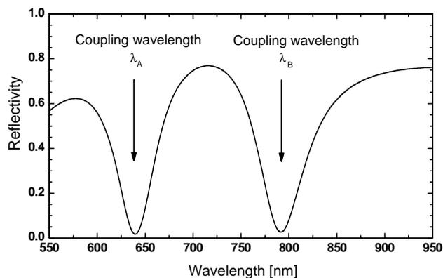
Fig. 7. Reflectivity in the WDMSPR sensing element as a function of wavelength. Sensing element—SF14 glass, metal layer—gold, thickness—55 nm, dielectric—aqueous medium, angles of incidence  $\alpha = 54.6^\circ$  and  $\beta = 52.5^\circ$ .
